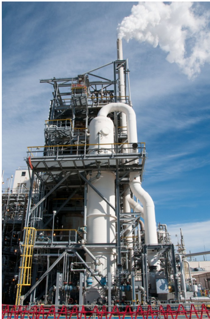
Figure 9. NRS Incinerator installed in 2011 to reduce emissions and allow increased production at the DuPont La Porte insecticide manufacturing facility.
