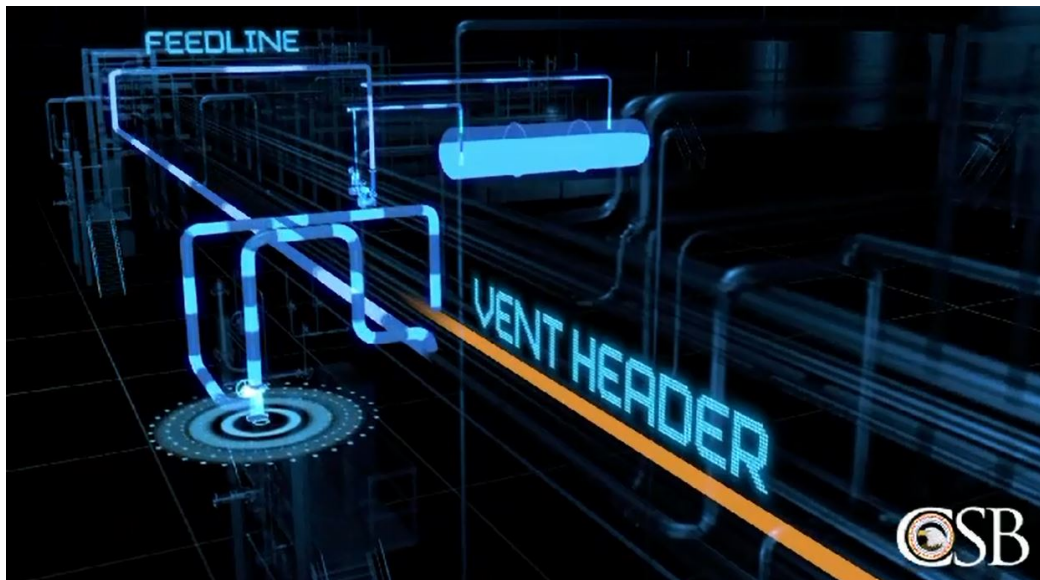
Figure 18. Snippet from CSB animation depicting the piping arrangement that allowed liquid methyl mercaptan from the feed line (blue) to flow into the waste gas vent header piping (orange).
