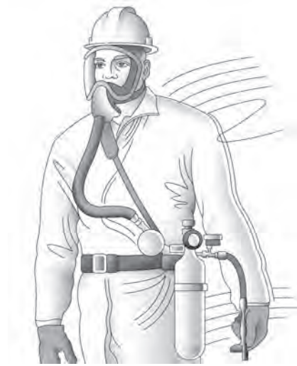
Full Facepiece Supplied-Air Respirator (SAR) with an auxiliary Escape Bottle APF=1,000 APF = 10,000 (if used in "escape" mode) Needs to be fit tested
