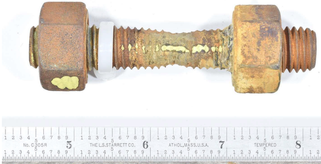
Figure 10. Post-incident examination photo of a corroded stud installed in the incident flange. (Credit: SES)
