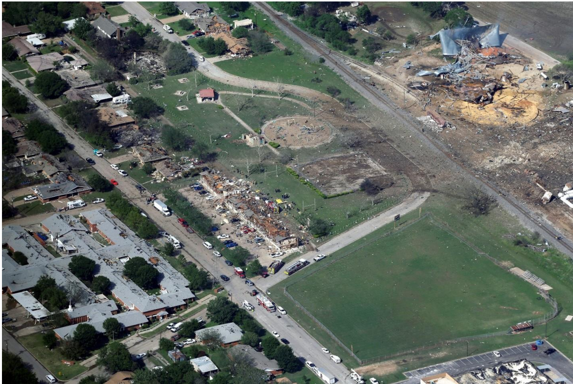
An ammonium nitrate storage depot at the West Fertilizer Company (at top right of picture) exploded on April 17, 2013, destroying an apartment complex (center) and 120 other buildings and killing 15.
