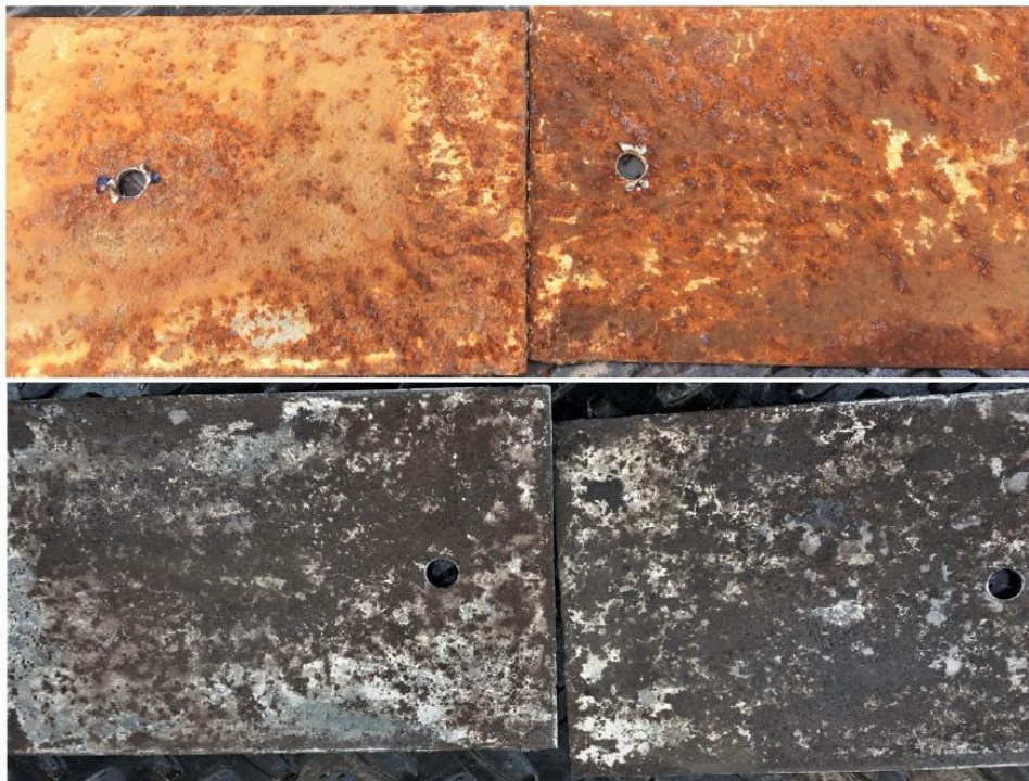
Figure 27. Photos showing passivation coupons that were used to determine the efficacy of the passivation operation for the Final Fractionator A overhead condensers. Before passivation (top) and 19 hours after passivation (bottom). (Credit: TPC)
