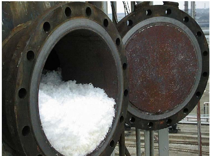
Figure 4. Popcorn polymer in a manway from an undisclosed facility (Credit: International Institute of Synthetic Rubber Producers Inc. [8, p. 261])
