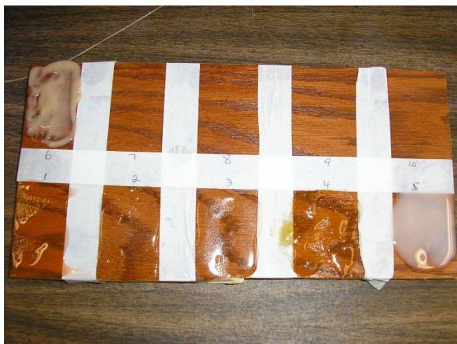
Figure 3-22. Wood Panel With Strippers Applied
