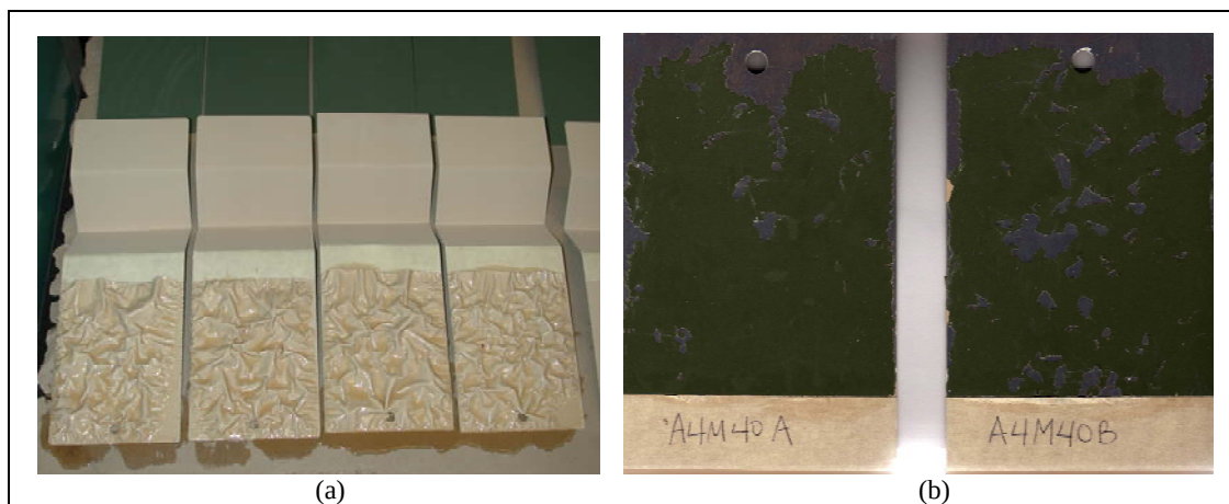
Figure 27. Crest Strip #28 began to lift the MIL-C-46168 within 5 min after application (a) and after 1.5 hr, all of the top layer was removed and some spots were removed down to the substrate (b).
