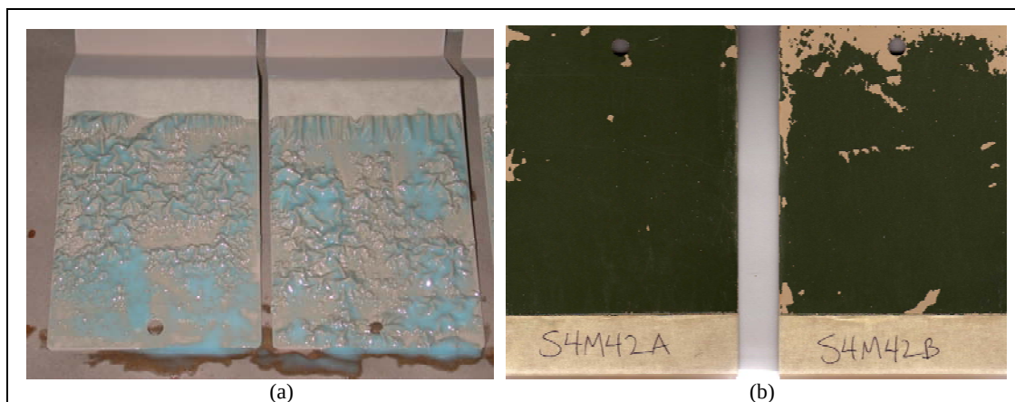
Figure 28. The D-Zolve 1220GEL began to show signs of paint lifting at about 40 min after application on MIL-C-46168 (a). The panels after the 1.5-hr dwell time (b). Nearly all of the first coating has been removed from panel a and about 90% of panel b.
