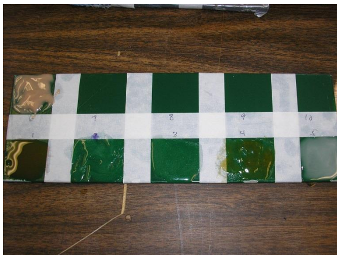
Figure 3-24. Green Metal Panel After Strippers Applied
