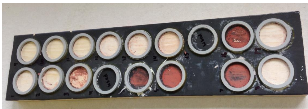
Figure 1: Wood coupon with ring gaskets after testing
