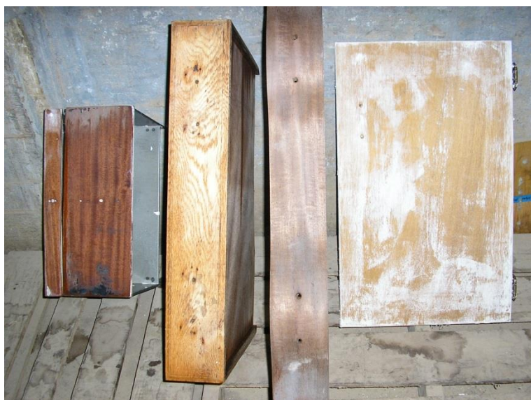
Figure 3-5. Items After Stripping With #B7 at Strip Joint.
