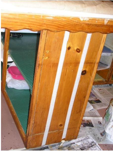
Figure 3-19. Panel #1 After Stripping
