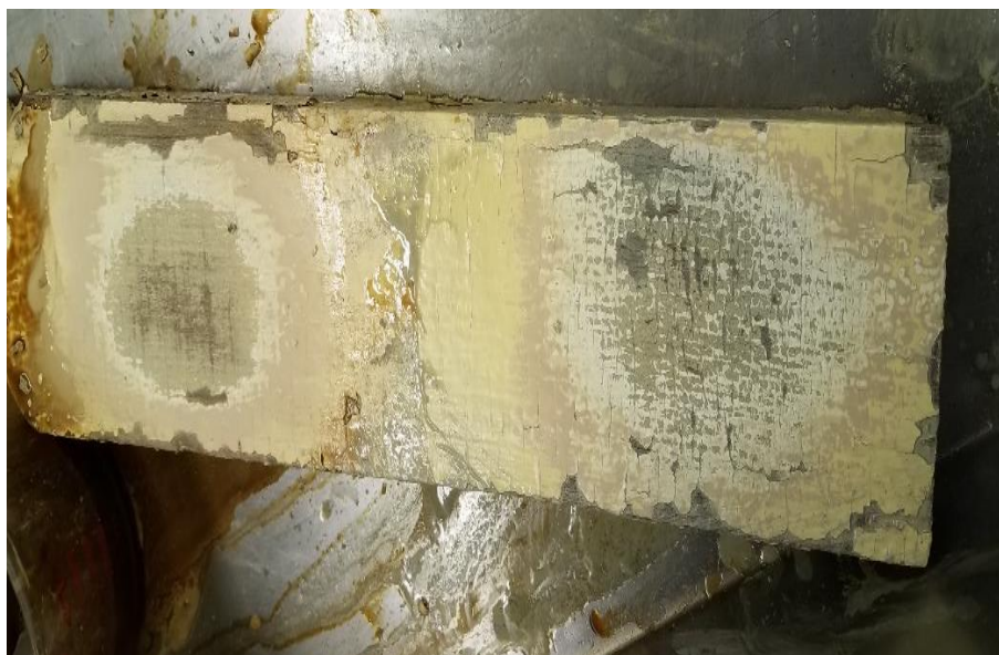
Figure 7: Testing results after 39 minutes (B7 on left side, Formulation #4 on right side)
