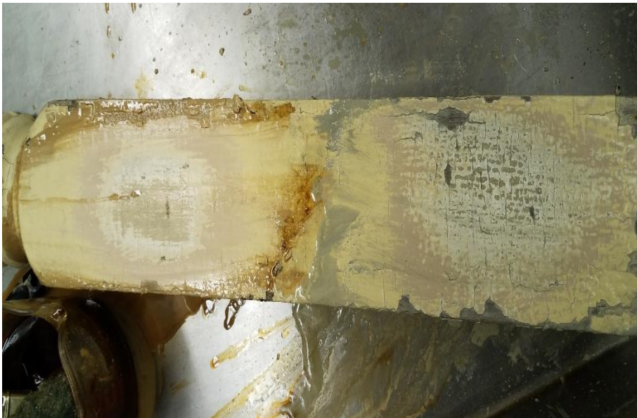
Figure 5: Testing results after 29 minutes (B7 on left side, Formulation #4 on right side)
