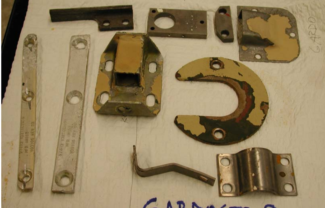
Figure 32. Stripping of miscellaneous parts after 30-min immersion in Gardostrip Q7900. A significant amount of paint remained, but parts were free of corrosion. One hundred percent of the paint was removed from one side of the C-flange.
